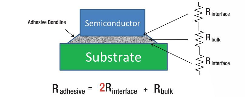
For effective heat transfer, the adhesive must have: Low bulk resistivity (high bulk ThK)
